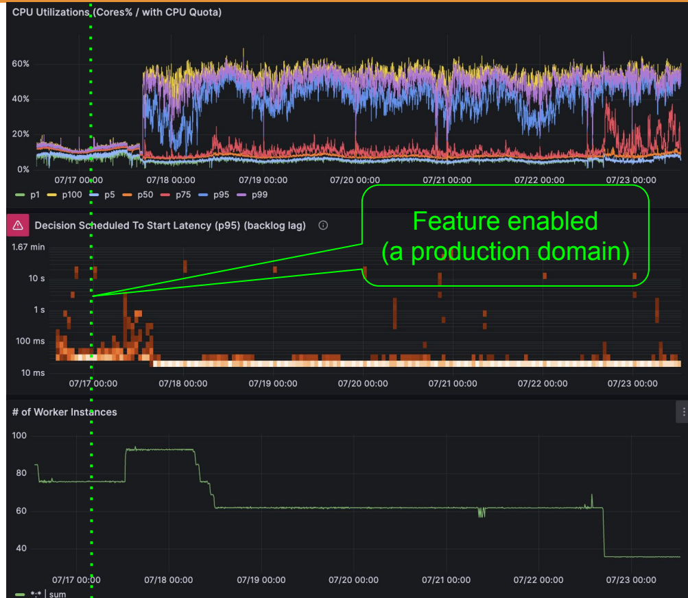
Figure showing the change in worker service CPU utilization, decision task latency and # of instances after the worker auto-scaling feature was turned on
