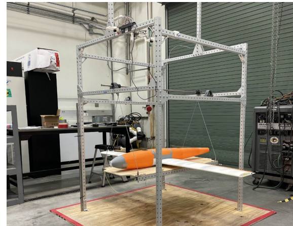
Moment of inertia rig for determining I_{xx} , I_{yy} , I_{zz}
