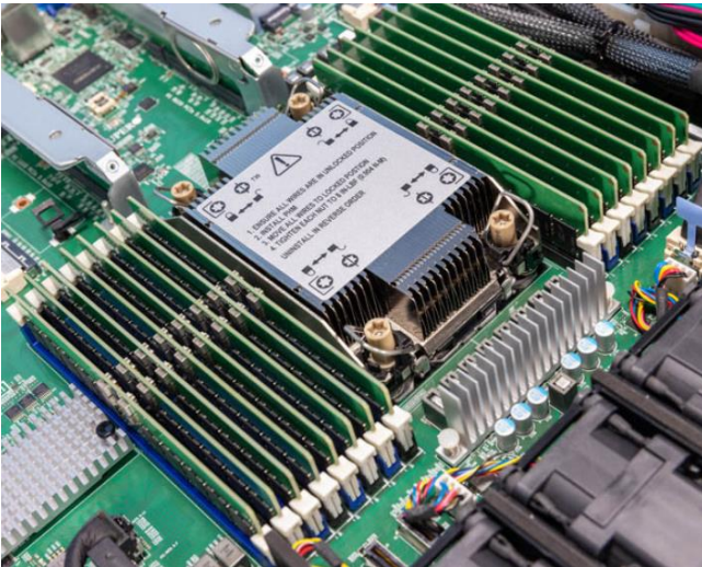
DRAM attached x86 server - Supermicro
